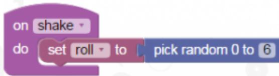
Having picked the random number, you will then need to display the number somehow. For this you will use the 5×5 LED matrix. However, the pattern displayed by the LEDs will depend on the value of the variable 'roll', so it will be necessary to introduce an 'if' block into our program. To do this, select the 'Logic' tab, and drag an 'if' block into place within the program as shown in the diagram below.
